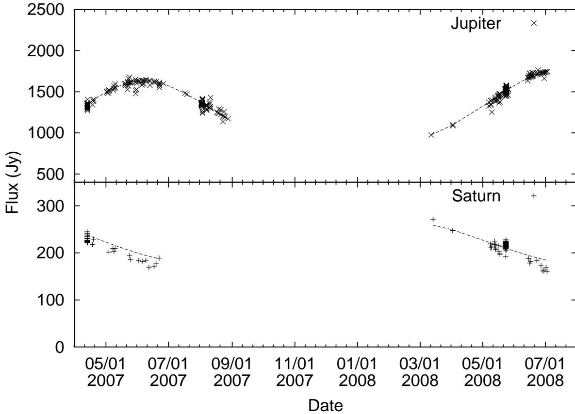
Fig. 6.— The recovered flux of our main calibrators, Jupiter (plus symbols) and Saturn (cross symbols) from the observations in 2007 and 2008. Data were calibrated by the first Jupiter measurement in the same night, or the nearest Jupiter measurement. The expected flux were plotted as dashed and solid lines for Jupiter and Saturn respectively.
