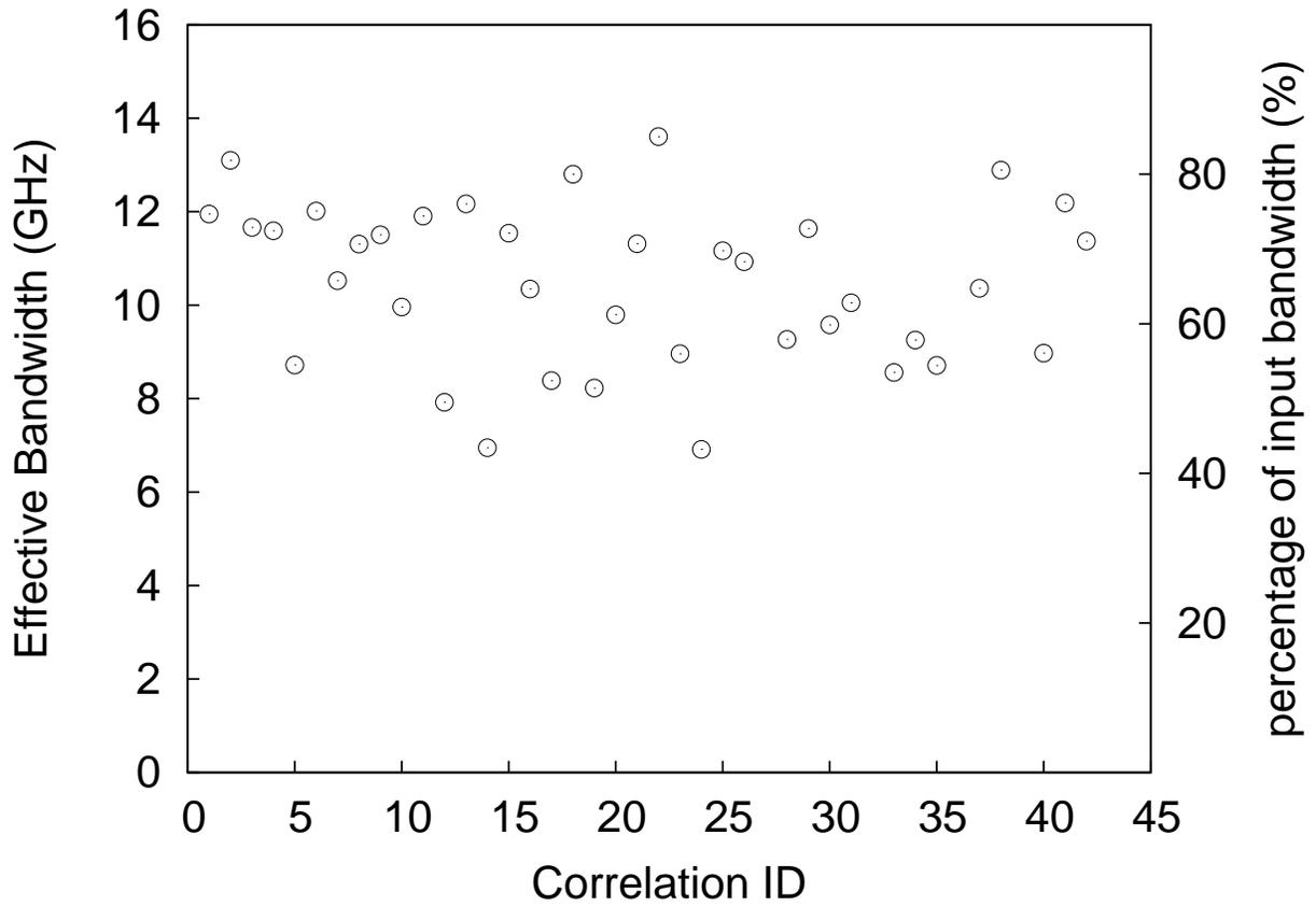
Fig. 2.— Effective bandwidths of the AMiBA correlators calculated from the bandpass displayed in Fig.1. The percentage is based on the nominal input bandwidth of 16 GHz.
