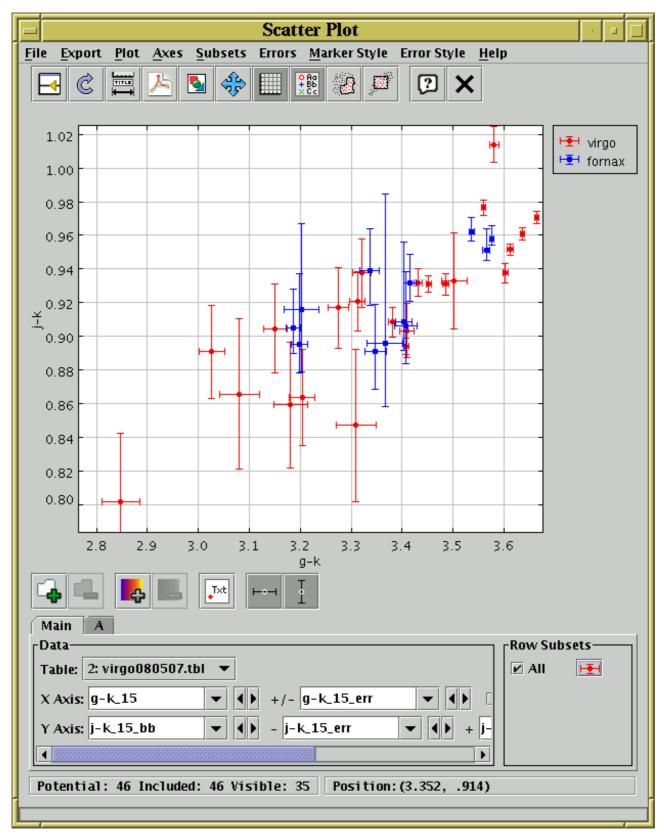
Plot window with symmetric X and asymmetric Y errors
